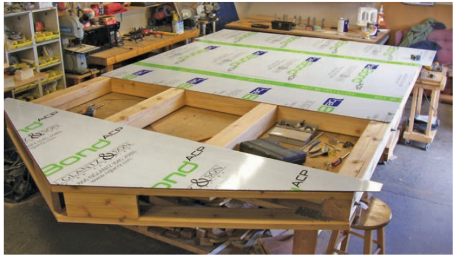
To ensure accurate layout, Richard and Christy Stetts made a mock-up with BeBond® aluminum-composite material.
